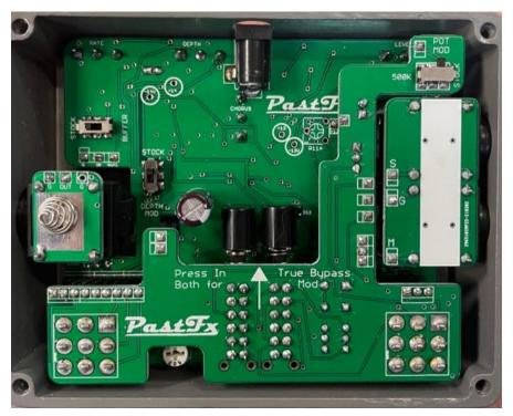
Note: In True Bypass Mode, Peak Level Indicator will not work when effect bypassed.
