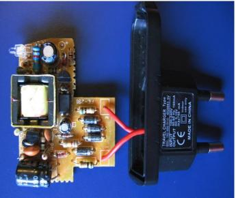
Both PSU's convert Mains AC to DC. The switch-mode is cheaper to manufacturer, produces less heat, but can introduce more noise than the Linear Supply. For Best Performance only use a quality Regulated, Isolated Linear power supply or professional high quality guitar intended switch mode.
